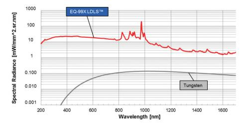
The spectral radiance (brightness) of the LDLS exceeds that of traditional Tungsten sources across the UV-Vis-NIR spectral range as shown in Figure 2.
